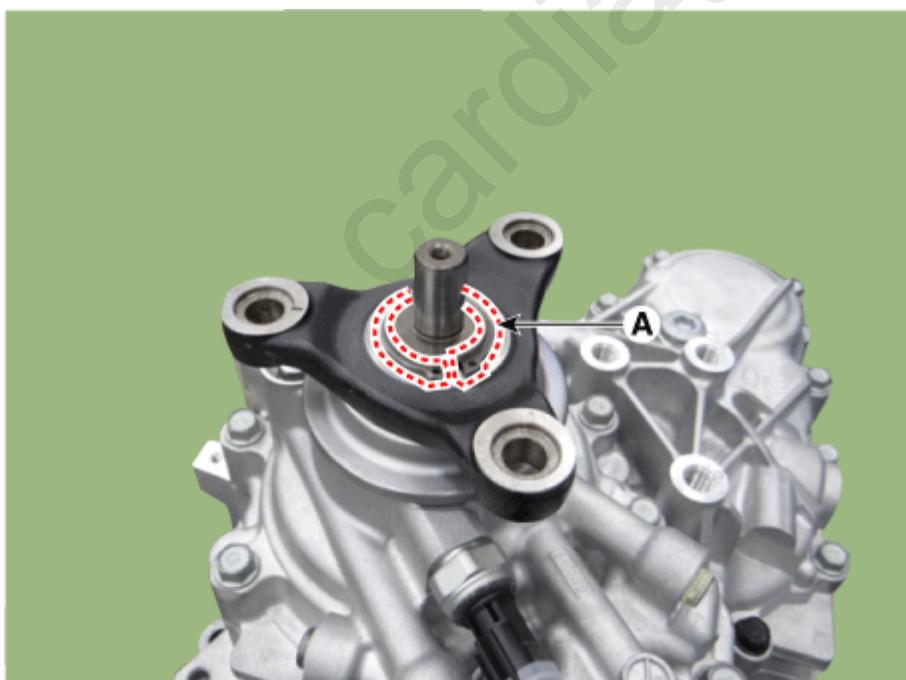
3. Remove the rear flange (A) using a gear puller.
