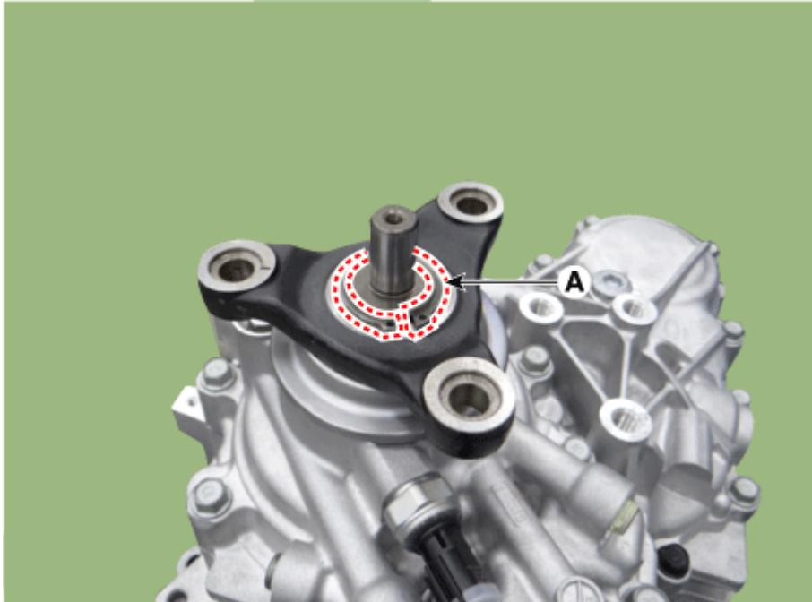
8. Install the rear propeller shaft assembly.
